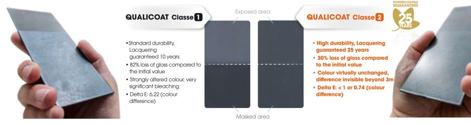
\*\*QUVB 313 test (standard 4892-3). The accelerated ageing chamber artificially reproduces the full solar spectrum. It simulates, in a few hours or weeks, the deterioration and damage caused by damage caused by solar irradiation and outdoor weathering over a period of several years compared to the loss of gloss of a Qualicoat Class 1 coating
