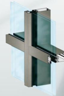
The grid look is obtained by placing horizontal and vertical caps on the exterior. These are clipped onto an aluminium clamping bar, which secures the glazing.
