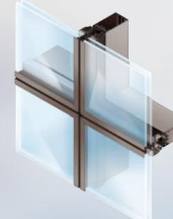
The VEP look is obtained by placing thermal bridge breakdown frames taking up an external aluminium glazing fillet that secures the glazing. They are assembled by mitre cut by means of serrated or crimped squares.
