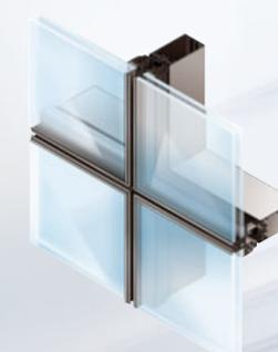
The VEC look is obtained by placing frames with non-edged glazing which do not show the aluminium structure on the outside. They are assembled by mitre cut by means of serrated or crimped squares.
