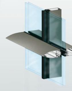
Placing horizontal caps and a double-hardness vertical seals on the outside creates the horizontal frame look. The horizontal cap is clipped onto an aluminium clamping bar that secures the glazing.
